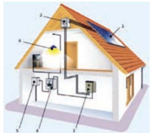
1. PV array; 2. PV array combiner / junction box; 3. Grid-tied inverter; 4. Import / Export meter; 5. Connection to the grid; 6. Load.
